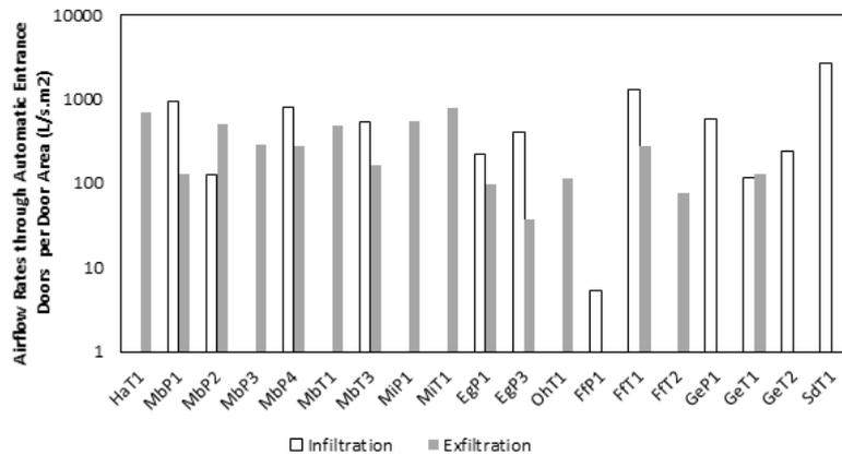
Figure 5. Calculated air infiltration and air exfiltration rates through the automatic entrance doors normalized by the door area.
