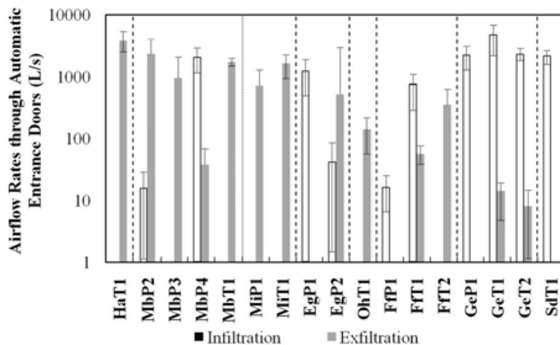
Figure 4. Calculated air infiltration and air exfiltration rates through the automatic entrance doors.
