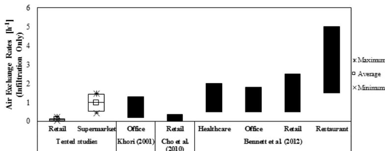
Figure 7. Calculated air exchange rates of air infiltration in retails and supermarkets compared to three existing studies.
