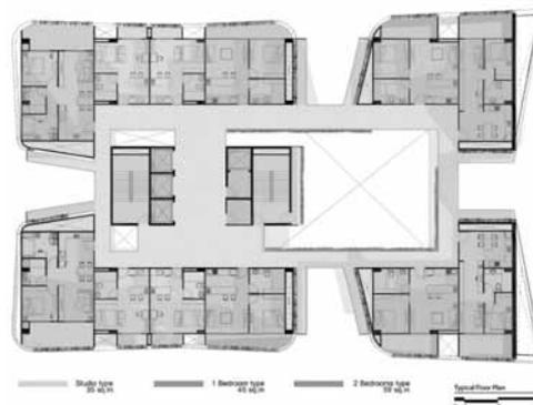
**Figure 15.** Floor plans of residential units on 6<sup>th</sup>-30<sup>th</sup> floor.
