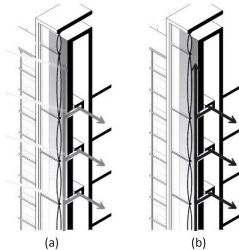
Another inspired idea for a sustainable design solution is the solar chimney, a type of passive solar heating and cooling system that uses the sun's heat to provide cooling by using the stack effect. Due to the extremely high light transmittance of ETFE, a solar chimney can be covered with this material as shown in the proposal for a refurbishment of a RMIT University building in Melbourne, Australia (Figure 3).
